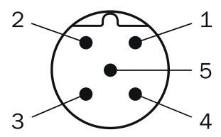
Male connector M12, 5-pin, A-coded
