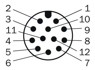
M12, 12-pin male connector, A-coded
