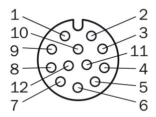
M12, 12-pin female connector, A-coded (I/O)  $\,$
